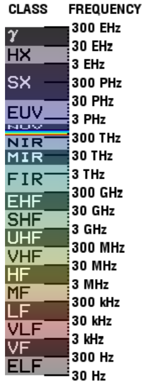
Fig 1. The Electromagnetic Spectrum (from the wikipedia article). Class designations are abbreviations for Extremely Low Frequency, Very Low Frequency, etc... Extreme High Frequency, Far Infra-Red, Near Ultra-Violet, X ray, and at the top of the scale, gamma rays. Notice that narrow band between NUV and NIR – this is the visible light band.
